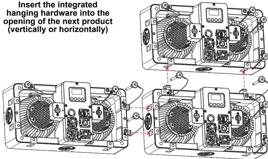
Insert the retaining pins to lock the products together
