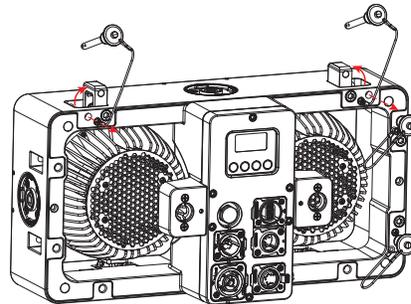
Insert the integrated hanging hardware into the opening of the next product (vertically or horizontally)
