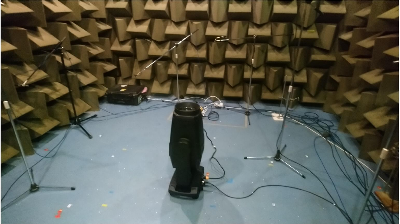
Figure 1 – unit under test mounted in the hemi-anechoic chamber at the University of Salford.
